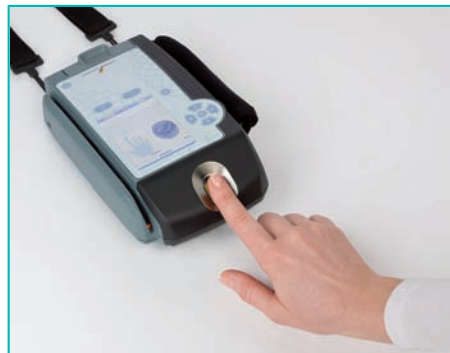
Mobile biometric scanner (Visotec) developed by the Bundesdruckerei for enrolment with German ID card.
